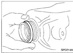
Reinstall all of the original side bearing adjusting shims on the carrier side, away from the ring gear.
