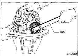
Remove side bearing adjuster with Tool. Tool number: ST32580000 (J34312)
