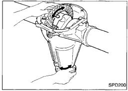
Hold companion flange steady and rotate the ring gear in both directions.
