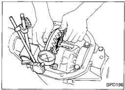
15. Measure ring gear-to-drive pinion backlash with a dial indicator. Ring gear-to-drive pinion backlash:
