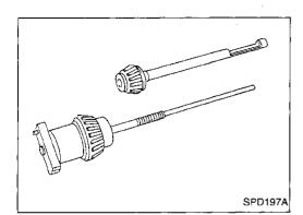
Front pinion bearing — make sure the J34309-3 front pinion bearing seat is secured tightly against the J34309-2 gauge anvil. Then turn the front pinion bearing pilot, J34309-5, to secure the bearing in its proper position.
