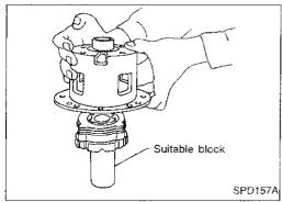
5. Install differential case A over side gear, discs and plates assembly.
