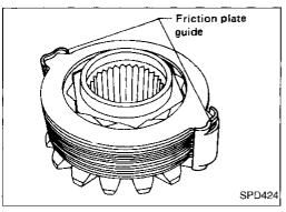
4. Install friction plate guides.
