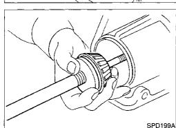
Assemble the front pinion bearing inner cone and the J34309-2 gauge anvil. Assemble them together with the J34309-1 gauge screw in the final drive housing. Make sure that the pinion height gauge plate, J34309-16, will turn a full 360 degrees. Tighten the two sections together by hand.
