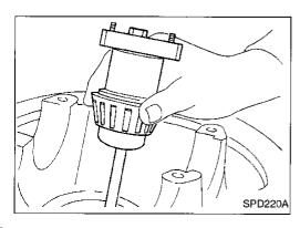
Remove the J34309 pinion preload shim selector tool from the final drive housing and disassemble to retrieve the pinion bearings.
