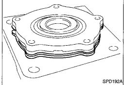
Place all of the original side retainer adjusting shims onto the side bearing retainer that goes at the ring gear end of the carrier.
