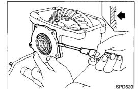
4. Mark side retainers for identification. Remove side retainers. Be careful not to confuse right and left side retainers and shims.
