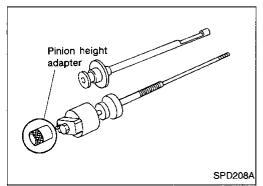
Place the J34309-14 pinion height adapter onto the gauge plate and tighten it by hand.
