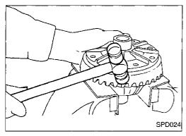
3. Tap ring gear off differential case with a soft hammer. Tap evenly all around to keep ring gear from binding.
