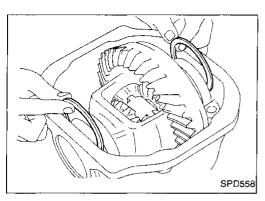
12. Insert left and right side bearing adjusting washers in place between side bearing and carrier.
