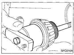
Place the pinion preload shim selector Tool gauge screw assembly, J34309-1, with the pinion rear bearing inner cone installed, into the final drive housing.
