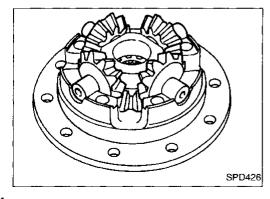
Install pinion mate gears and pinion shaft to differential case B.
