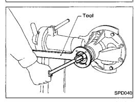
8. Temporarily tighten pinion nut until there is no axial play.
