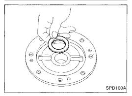
10. Install side gear thrust washer to differential case B.
