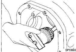
Install the pinion rear bearing inner cone into the final drive housing. Then place the pinion preload shim selector Tool, J34309-1, gauge screw assembly.
