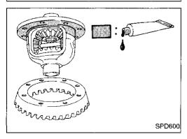
Apply locking agent [Locktite (stud lock) or equivalent] to contacting surfaces of ring gear and differential case, then place differential case on ring gear.
