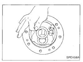
4. Install side gear thrust washer to differential case A.
