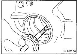
4. Assemble the front pinion bearing inner cone and the J34309-2 gauge anvil together with the J34309-1 gauge screw in the final drive housing. Make sure that the pinion height gauge plate, J34309-16, will turn a full 360 degrees, and tighten the two sections together by hand.
