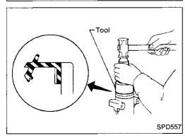
Apply multi-purpose grease to cavity at sealing lips of oil seal.
