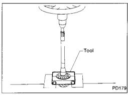
10. Remove pinion rear bearing inner cone and pinion height adjusting washer.
