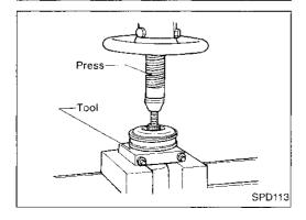
5. Remove center bearing using Tool and press. Tool number: ST30031000 (J22912-01)
