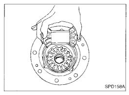
6. Install pinion mate gears, pinion shaft and thrust block to differential case A.
