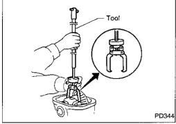
Remove the carrier from the final drive housing. Save the selected preload washers for later use during the assembly of the final drive unit.
