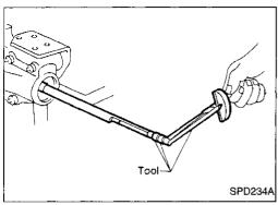
Measure the turning torque at the end of the J34309-2 shaft using Tool.
