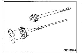
Front Pinion Bearing — make sure the J34309-3 front pinion bearing is secured tightly against the J34309 gauge anvil. Then turn the front pinion bearing pilot J34309-5 to secure the bearing in its proper position.
