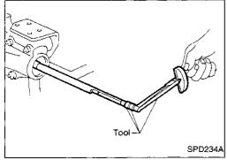
Measure the turning torque at the end of the J34309-2 gauge anvil using Tool.
