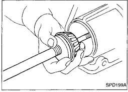
4. Install the J34309-2 gauge anvil with the front pinion bearing into the final drive housing and assemble it to the J34309-1 gauge screw. Make sure that the J34309-16 gauge plate will turn a full 360 degrees, and tighten the two sections by hand.
