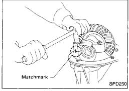
3. Remove side lock fingers and side bearing caps.
