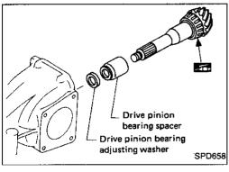
Place drive pinion bearing spacer, pinion bearing adjusting washer and drive pinion in final drive housing.
