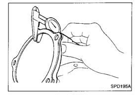
Record the correct, selected total thickness of the side retainer adjusting shims, and remove the carrier and bearings from the final drive housing. Save all shims for later re-use.
