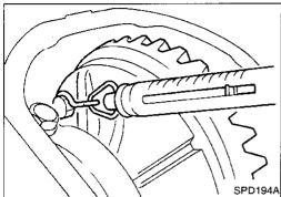
7. Measure the turning torque of the carrier at the ring gear retaining bolts with a spring gauge, J8129.
