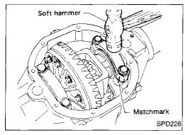
14. Align mark on bearing cap with that on gear carrier and install bearing cap on gear carrier.
