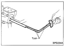
Measure the turning torque at the end of the J34309-2 gauge anvil using Tool.
