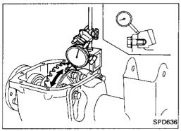
18. Check runout of ring gear with a dial indicator.
