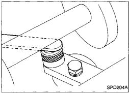
Select the correct standard pinion height adjusting washer thickness. Select by using a standard gauge of 3 mm (0.12 in) and J34309-101 feeler gauge. Measure the distance between the J34309-11 pinion height adapter including the standard gauge and the arbor.
