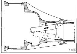
Remove pinion front and rear bearing outer races with brass drift.
