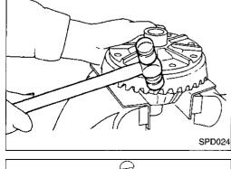
4. Punch off pinion mate shaft lock pin from ring gear side. Lock pin is calked at pin hole mouth on differential case.
