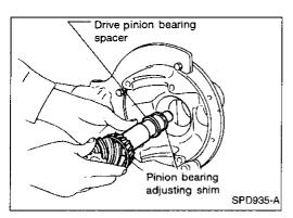
6. Install drive pinion bearing spacer, pinion bearing adjusting shim and drive pinion in gear carrier.
