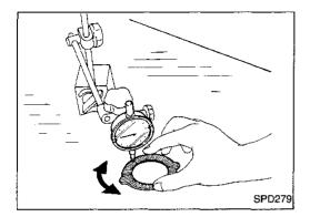
3. Check friction discs or plates for warpage.
