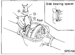
13. Drive in side bearing spacer with Tool. Tool number: KV38100600 (J25267)
