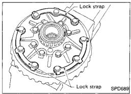
2. Spread out lock straps and loosen ring gear bolts in a criss-cross fashion.
