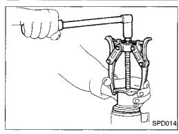
Remove pinion nut with Tool. Tool number: ST38060002 (J34311)
