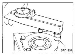
4. Install both bearing retainers onto the final drive housing and torque the retainer bolts.
