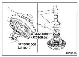
Reinstall the carrier side bearing using Tools J25805-01 and J8107-2. Press on the bearings.
