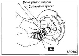
Install drive pinion washer, collapsible spacer and drive pinion in gear carrier.
