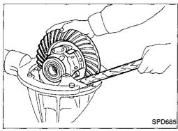
5. Remove differential case assembly with a pry bar.
