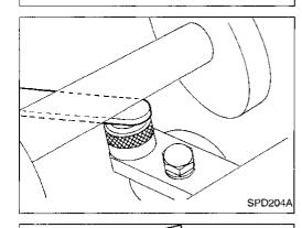
10. Select the correct standard pinion height adjusting washer thickness by using J34309-101 feeler gauge. Measure the gap between the J34309-14 pinion height adapter and the arbor.
